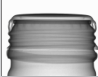
▲Aluminum bottle with cap Taken with the C7876 and microfocus X- ray source
