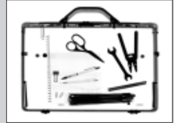
▲Interior of bag Taken with an X-ray line scan camera
